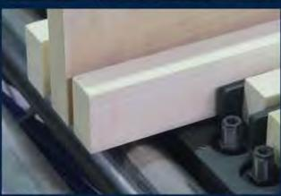
Heavy duty air operated stops resist dust and debris while maintaining quick and consistent operation.
