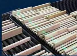
Scanning is based on line lasers at high angles being read from USB based array cameras. As many as 34 staves are measured at any time for each panel solution. Final solutions within +/- 050" up to 40" wide panels. The final stave groups are kept together and fed to a customer supplied glue wheel.
